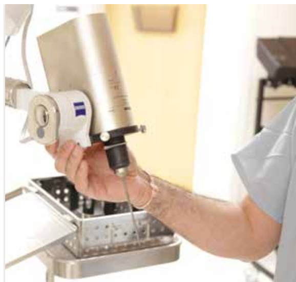
ABOVE: The IORT device delivers radiation from a miniature accelerator tip attached to a robotic arm.
